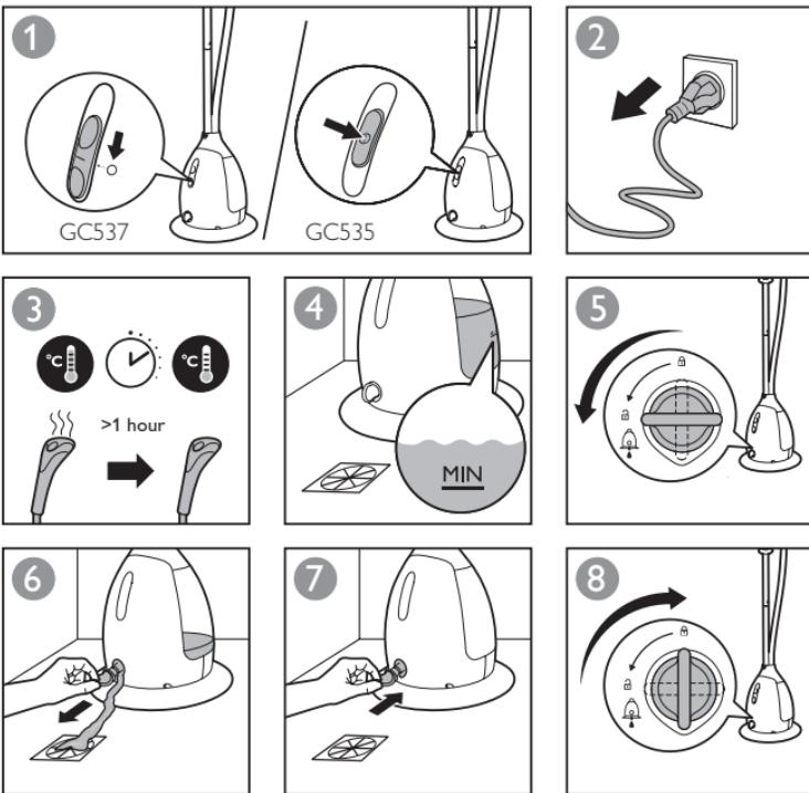
**EN** To maintain optimal steam performance, it is important to remove scales and impurities inside the appliance regularly. Therefore, it is recommended to perform the easy rinse calc-clean process at least once a month. Before you start calc-clean, make
