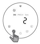
With the light sensor, the control panel can automatically turn on, turn off or dim according to the ambient light. The control panel will be off or dim when the ambient light is dark. You can touch any button to wake up all lights. Then, if no further operation, all lights will be off or dim again to match with the ambient light.
