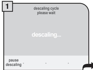
The machine begins to dispense the descaling solution through the hot water spout. The dispensing occurs at preestablished intervals, in order to allow the solution to be more effective.
