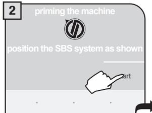
Press the display once and the machine will begin priming the water circuit.
