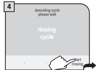
Rinse the machine circuits by pressing "start rinsing".
