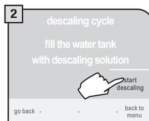
When in the descaling menu, the message "fill the water tank with descaling solution" appears on the display.
