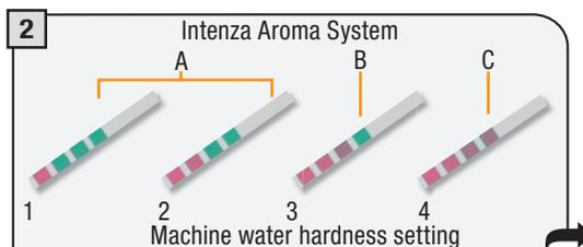
Check the water hardness level obtained from the test.
