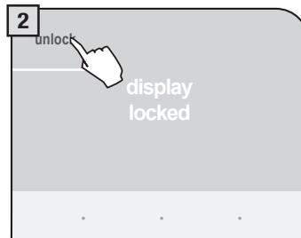
To reactivate the display, press "unlock" on the lower right-hand corner and then (within two seconds) "unlock" in the upper left-hand corner (this button appears only after having pressed the previous button).
