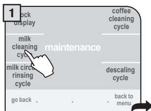
Select the function by pressing the “milk cleaning cycle” button.
