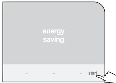
To activate the machine, press "start". After having performed the function diagnostics and the heating up phase, the machine is once again ready for use.
