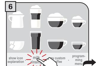
The "milk rinsing" icon will flash once the machine is done dispensing in order to clean the milk circuit. Press the "milk rinsing" icon to clean the internal milk circuit.
