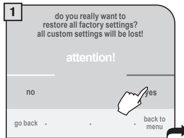
If "yes" is selected, a subsequent confirmation by inverted switch buttons is requested to be sure that you want to perform the reset.
