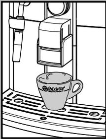
Manually move the dispensing spout up or down to adjust its height by placing your fingers as shown in the figure.
