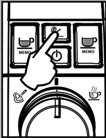
22 Hold the “MEMO” button pressed for 6 seconds to reset the machine and cancel the descaling alarm signal. The light “MEMO” turns off.
