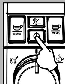
At this point the button “MEMO” is programmed; each time it is pressed and released, the machine will brew the same amount of coffee that was just programmed.
