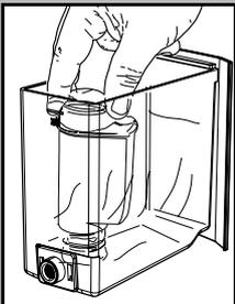
Put the water filter into the empty tank. Press it until its limit stop.
