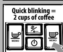
**i** To brew 2 coffees, the machine automatically grinds and doses the correct amount of coffee. Brewing two coffees requires two grinding cycles and two brewing cycles, which the machine carries out automatically.
