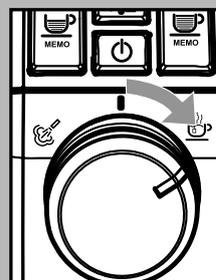
19 Turn the selector switch clockwise to set it to the "☕" position.
