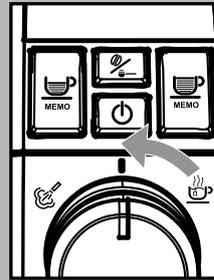
9 Dispense water until the no water signal is displayed, then turn the selector switch counter-clockwise to set it to the “☕” position.
