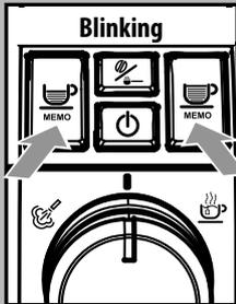
**i** Occasionally, after turning the selector switch, hot water may not be dispensed and the buttons will start blinking. Simply wait until the end of the warm-up phase so that hot water can be dispensed from the Pannarello.
