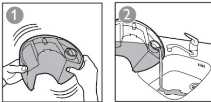
**EN** Always empty the water tank after use, to prevent scale build-up. Rinse the water tank to remove any deposits.
