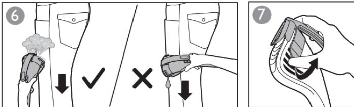
**EN** **Caution:** Do not attach or detach the pleat maker while the steam is on or the steamer head is hot.
