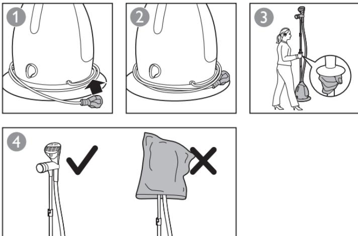
**EN** Always store the appliance in a place with good ventilation. Do not cover the steamer head during storage.
