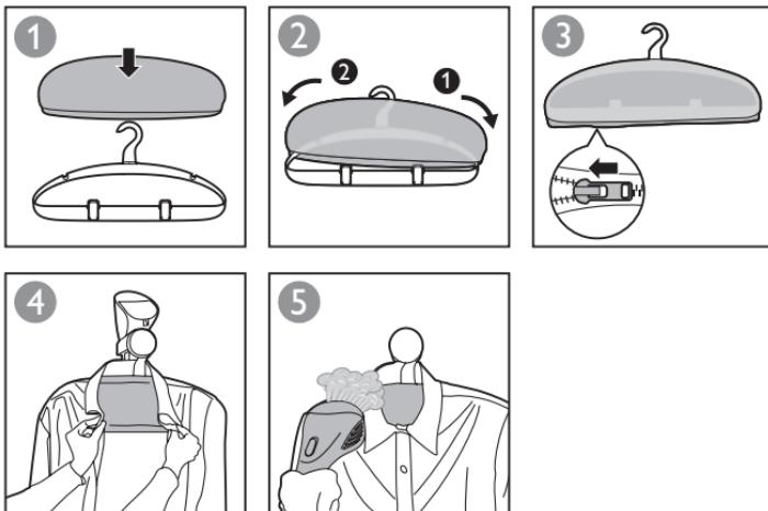
**EN** You can remove wrinkles from the shoulder parts easier with Shoulderfit Hanger. The special 3D fabric pad in the ShoulderFit Hanger provides additional support so you can press the steamer head against the pad for better and faster result.
