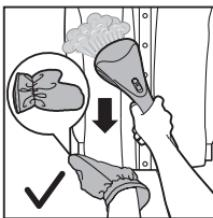
**EN** Do not use your bare hand as support when you are steaming. To avoid burns, wear the glove provided on the hand with which you are holding the garment.
