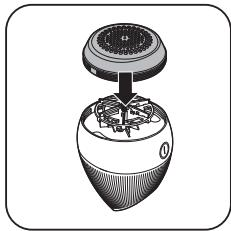
**12** Attach and screw the lid back onto the appliance.
