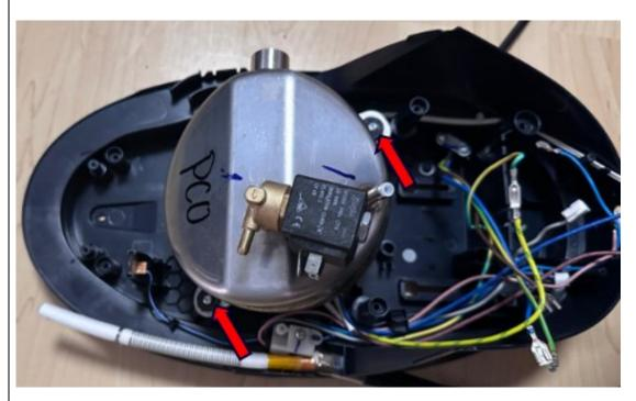
Step 16: To remove Powercord (27) unscrew Q (2x) from Stand Bottom Assy (3) as shown
