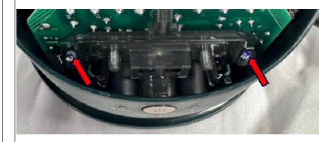
Step 12: Unplug all the quick connectors from Power PCBA (33), E-valve (110) & Pump Assy (11) as shown
