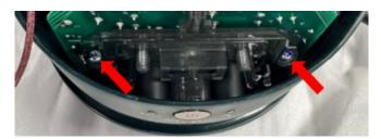
C. Ensure the Rinse outlet tube rib is aligned as shown below, also the rib is aligned with the Stand top Assy slot as shown
