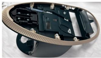
Step 10: Remove the Rinse outlet tube from Stand Bottom Assy (3) and Boiler Assy (7) as shown
