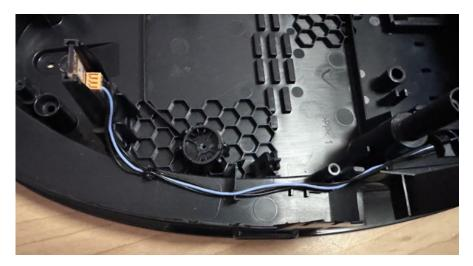
Step 2: Assemble Hosecord Assy (107) using screw R (1x) **Torque 9 ±1** Kgf. to the Stand Bottom Assy (3) as shown
