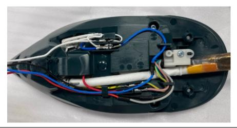
E. Assemble the housing to the cover as shown, then place the wire seal as shown Note: Ensure before assembling the housing rubber bung should be placed on housing as shown
