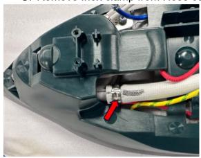
CAUTION: ENSURE DO NOT DAMAGE THE HOSE CORD TUBE WHILE REMOVING INOX CLAMP
