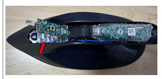
I. Fasten screw B, C, & D (Each 1x) Torque 5 ±1 Kgf. Iron PCBA to the housing as shown
