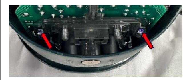
Step 11. Assemble the Rinse outlet tube to Boiler Assy, ensure the rinse outlet tube orientation as shown
