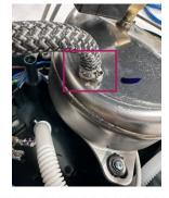
CAUTION: ENSURE DO NOT DAMAGE THE BRAIDED TUBE WHILE REMOVING INOX CLAMP
