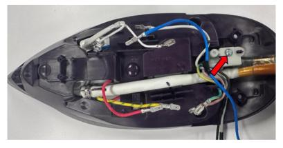
G. Remove Inox clamp from Hose cord tube and remove the hose cord tube
