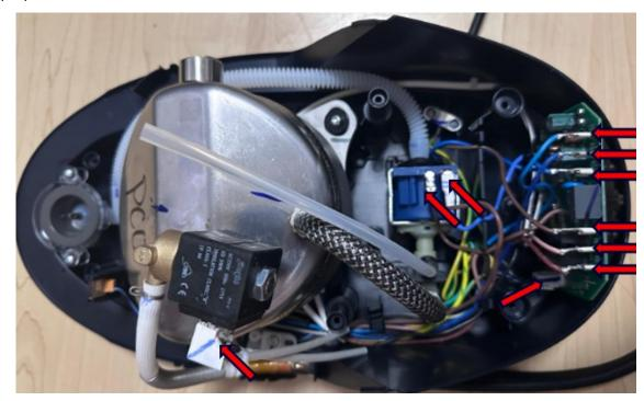
Step 13. Remove the Braided tube and Hose cord tube from Boiler Assy (7) as shown. Caution: Ensure do not damage the braided tube while removing the inox clamp.
