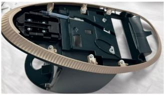
Remove all the wires and quick connectors from PCBA & Pump Assy as shown
