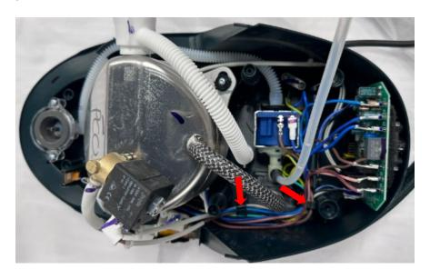
F. Connect the De-air tube to the hose connector and dress the tube as shown
