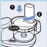
**1** Mount the bowl on the food processor by turning the handle in the direction of the arrow until you hear a click.
