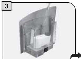
3 Fill the tank with fresh drinking water. Let the water filter soak in the full tank for 30 minutes for correct initialization.
