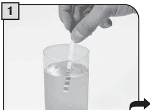
Immerse the water hardness tester provided with the machine in water for 1 second.
