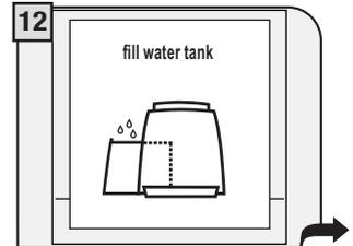
Once the rinse cycle is finished the following screen appears. Remove the tank, install the "Aqua Prima" water filter again (if desired) and fill it with fresh drinking water.
