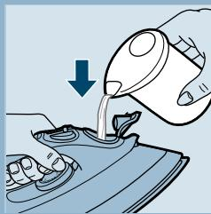
If the tap water in your area is very hard, we advise you to mix it with an equal portion of distilled water; or to use distilled water only.
