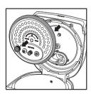
To assemble the detachable inner lid, fully attach it to the top lid, and then screw the nut around the temperature controller clockwise.
