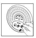
To assemble the floater, put the thin end of the floater into the hole on the lid (fig.(1)), and assemble the rubber ring around the floater (fig.(2)).
