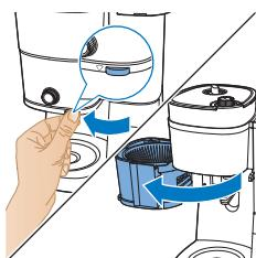
2 Open the filter holder to access the ground funnel chute.
