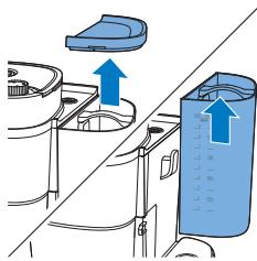
1 Open the lid of the water reservoir and lift the tank from the appliance.
