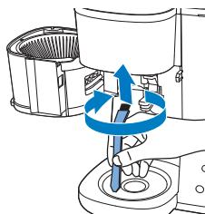
7 Use a brush to remove any coffee grounds or residue that may have accumulated in the chute.
