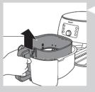
**2** Remove the basket by lifting the handle.
