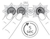
Press and hold the Espresso, Lungo and Intensity boost buttons simultaneously for 5 seconds until all leds start to flash fast to show that the machine has been reset to factory settings.
