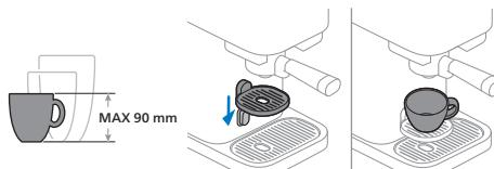
Place a smaller cup (with a height of up to 90 mm) on the cup platform.
