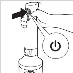
**6** Press the On/off or TURBO button and let it operate until all ingredients are cut.
