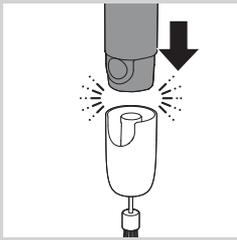
**2** Attach the whisk coupling unit to the motor unit (“click”).
