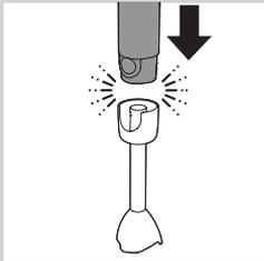
**1** Attach the blender bar to the motor unit (“click”).
