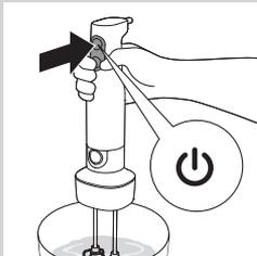
**6** Switch the appliance on by pressing the On/off button or the TURBO button.
