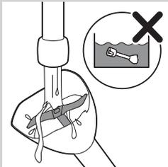
**9** For easy cleaning, rinse the bar immediately after use with hot water. Do not immerse the bar completely in water.
