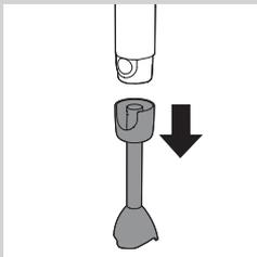
**8** Remove the blender bar by pressing the release button.
