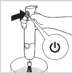
**6** Switch the appliance on by pressing the On/off or TURBO button.
